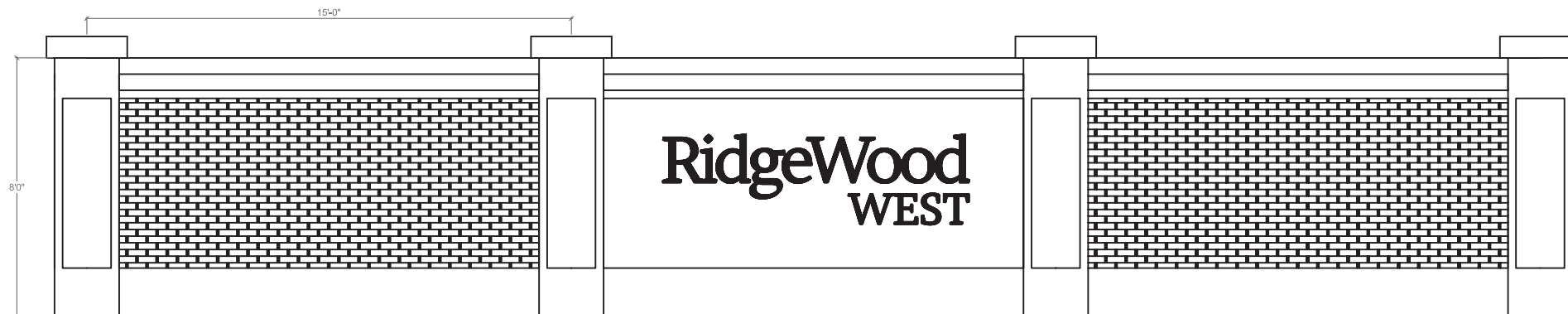
4 Rear Yard Concrete Fence Elevation - Typ. 1BW Concrete Fence Design - NTS
