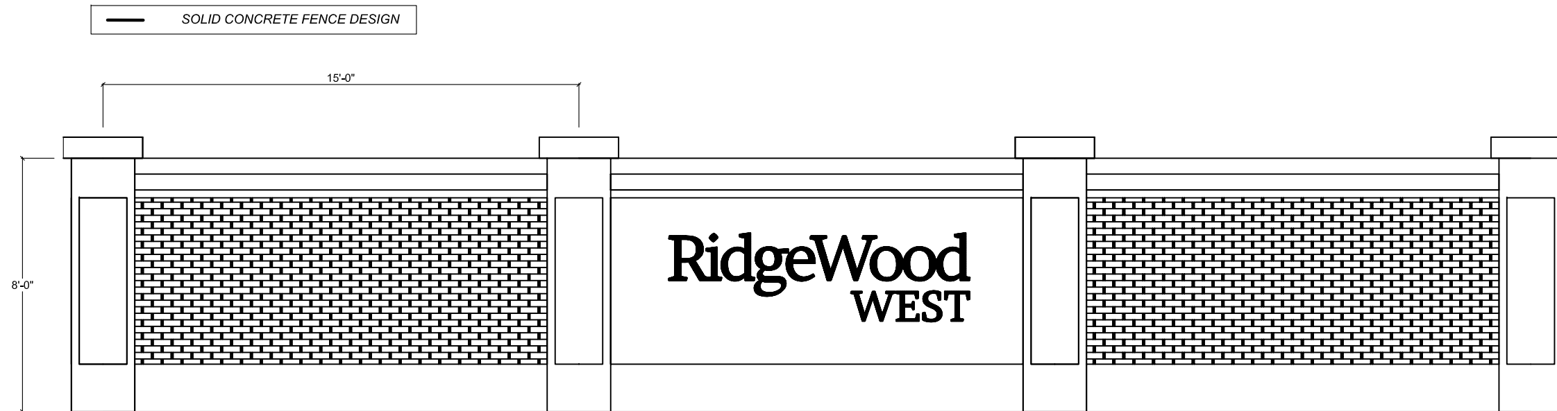
2 Rear Yard Concrete Fence Elevation - Typ. 2AW Solid Concrete Fence Design - NTS
